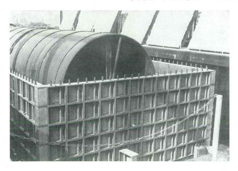
This furnace measuring 7.2 metres wide  $\times$  7.2 metres high and 25.8 metres long inside was constructed alongside the dock in sections with stainless steel encased insulation blocks. It was fired by natural gas using 8-625,000 K. cals/hour high velocity burners. Readings of gas consumption over the first three heat treatments indicated a thermal efficiency in excess of 40% for loads varying from 100 tons to 250 tons.
